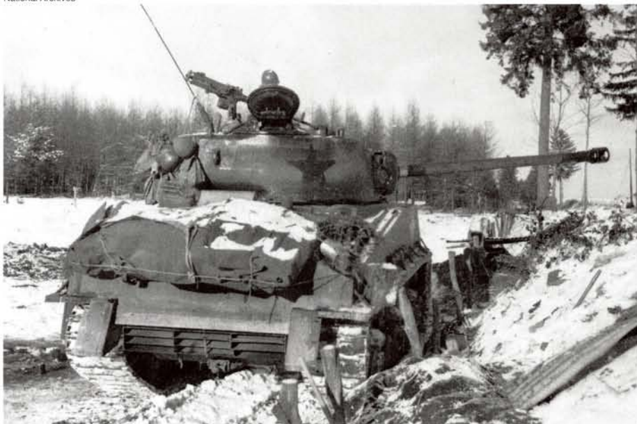
Its star insignia painted dark, an American M4 Sherman tank takes up a position in the snow near the town of Bastogne, Belgium, during the Battle of the Bulge. Note the high-velocity 75mm cannon that replaced the less potent main weapon on the earlier Sherman models. RIGHT: Captain James Leach served as John Parks's company commander and inspected the tank in which Parks died following the battle at Flatzbourhof.
